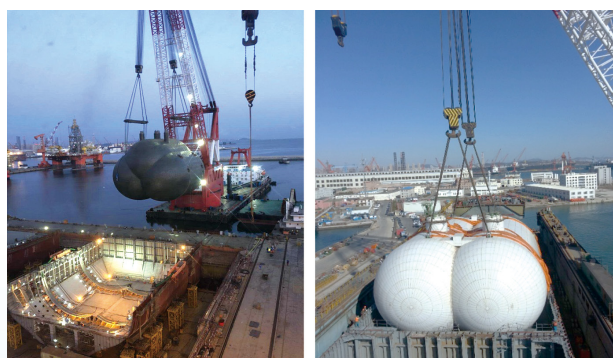
Lifting of Type C independent tank
